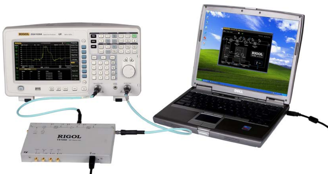
Figure 7 Test the Band-pass Filter Characteristics
